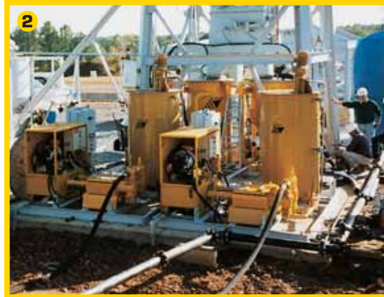
1) Channel Tunnel Rail Link-CTRL Contract 240: PLC controlled backfill plant with ZMP 712 and ZMP 725 grout pumps. London.
